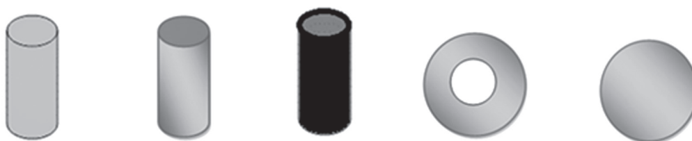
Figure 5. Different solid-conductor shapes and materials (Ag pellet, Ag/AgCl pellet, rubber pellet, Ag/AgCl ring, Ag/AgCl disc respectively).
