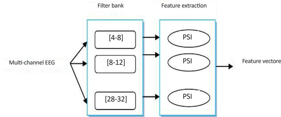
Figure 4. Block diagram of applied filter bank
