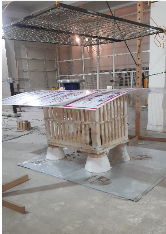
Figure 1. The monkey's cage under a uniform electrical field of 3 kV/m
