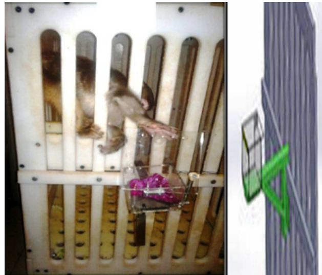
Figure 2. A plexiglass transparent container designed to perform a visual learning test and the cage prepared by teflon
