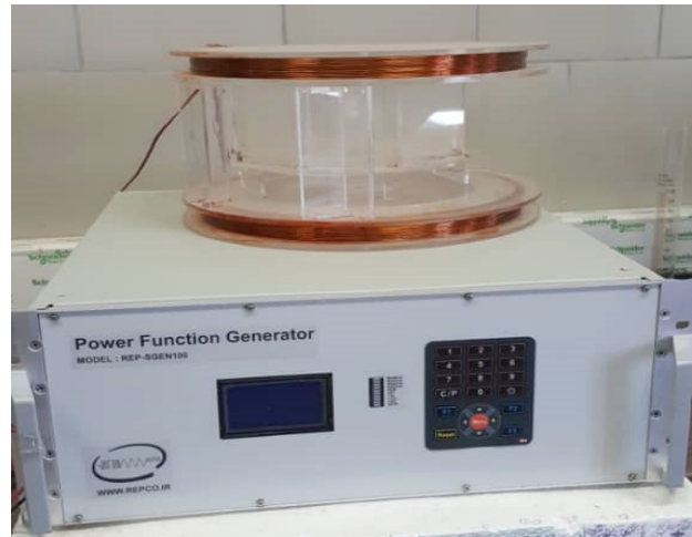
Figure 1. Schematic view of Helmholtz coils
